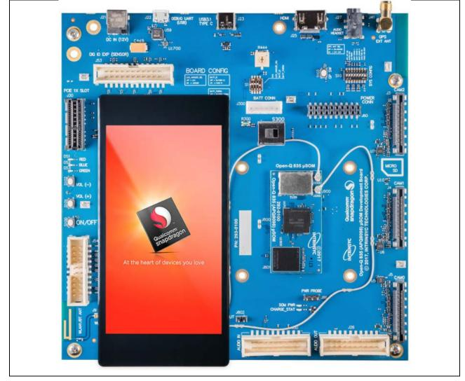
Figure 1 Assembled Open-Q 835 µSOM Development Kit
