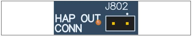
Figure 25 J802 Haptic Driver Header
